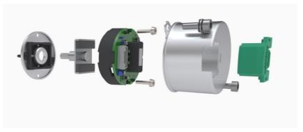
This kit version contains 4 main parts to be assembled from left to right side: shielding, magnet, carrier with PCB and housing.
