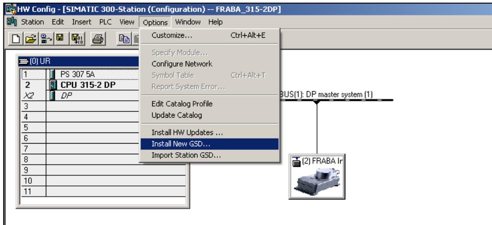
After the successful installation of the GSD file the FRABA inclinometer can be found in the hardware catalogue under „PROFIBUS-DP“ – „Additional Field Devices“ – „General“.
