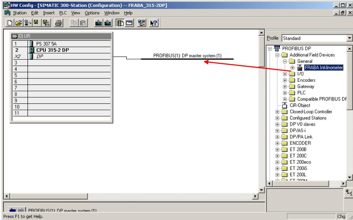
After inserting the Profibus master system in the hardware configuration (“Insert” – “Master System”) the FRABA encoder can be chosen from the hardware catalogue and added to the Profibus network: Select the device “FRABA Inclinometer” and drag it with the mouse to the network (or choose the network and double click the “FRABA Inclinometer”).
