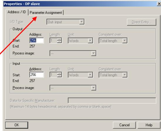
Device Parameter can be set in the following dialog box. For a detailed description of the parameters please refer to chapter 3.3.
