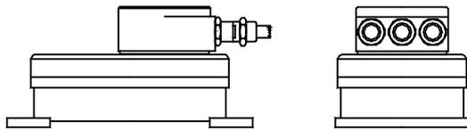
The device cannot be used in the following mounting positions:
